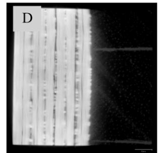
*$\mu$ -X-ray scans revealing the brick structure of laminate (light) and the pore microstructure of the wedge-shaped piece of balsa (dark with light spots).*
